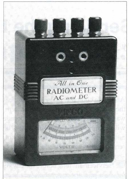
The Pifco ‘All in One’ Radiometer. Armed with such a device and one’s senses of smell and touch, it was surprising what could be handled in the way of early radio servicing
