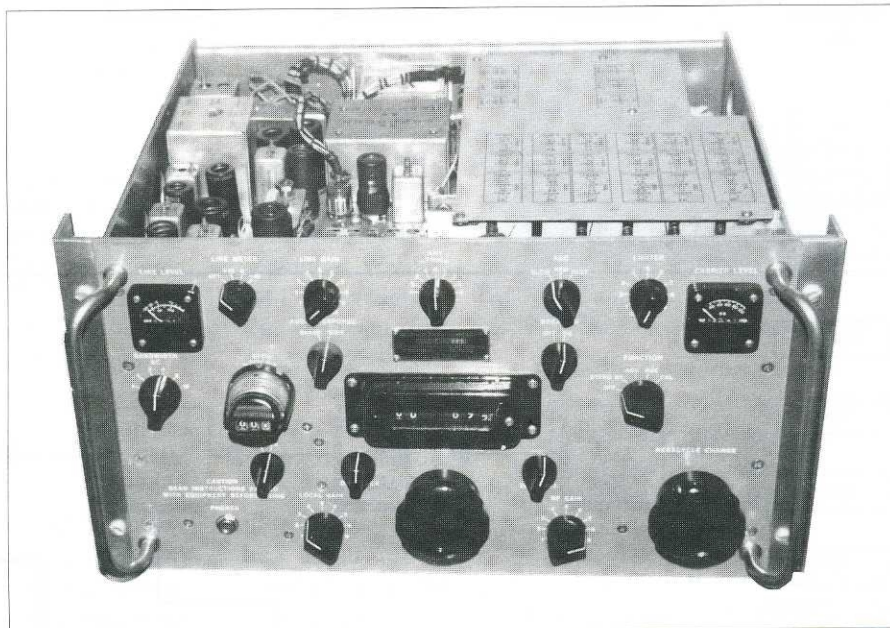
One of the author's R390A receivers, with the cover-plate carrying coil idents in position. This receiver is fitted with a digital read-out for the BFO Pitch control
