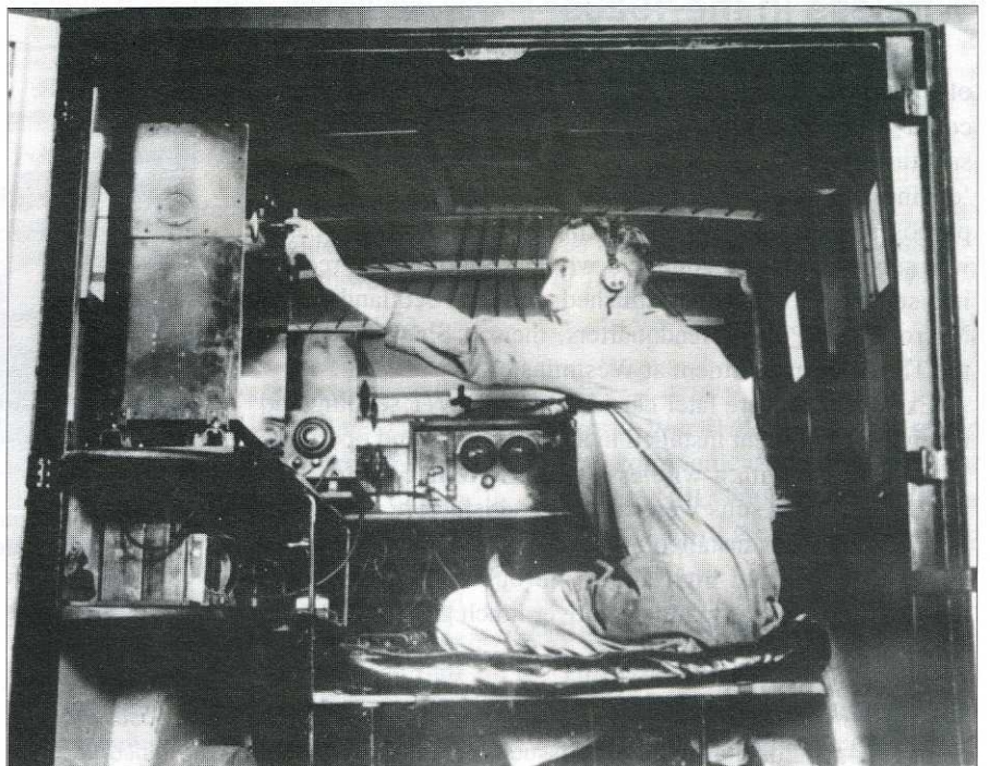
Photo 2 - Interior of a CID wireless van equipped with a transmitter and receiver. The aerial was a network of parallel wires in the roof. An engineer is tuning the transmitter prior to operation
